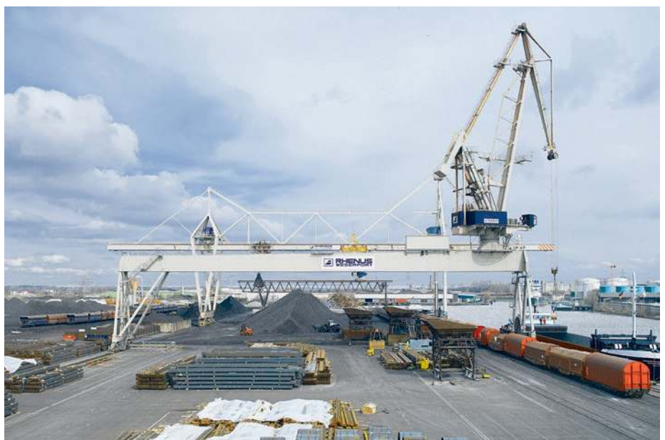
↑ Tukan with an asymmetrical gantry
