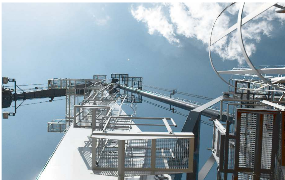
↑ Maintenance-friendly: even the boom is accessible via stairs
