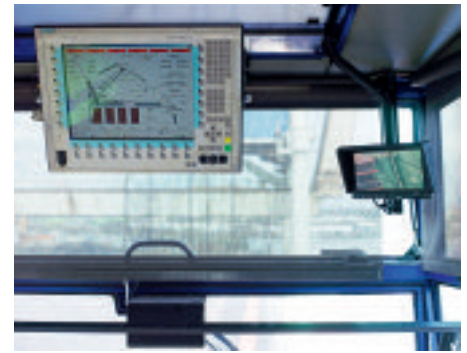
↑ Visualisation of crane dates via the crane management system
