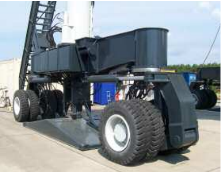
↑ Mobile travel mechanism with integrated propping system
